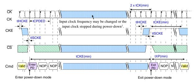
Input clock frequency can be changed or the input clock can be stopped or floated during power-down, provided that upon exiting power-down, the clock is stable and within specified limits for a minimum of 2 clock cycles prior to power-down exit and the clock frequency is between the minimum and maximum specified frequency for the speed grade in use.
