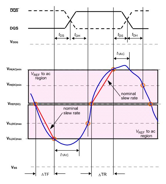
Setup Slew Rate Falling Signal =
