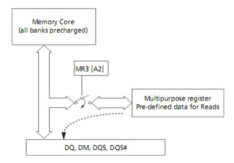
Fig. 1: MPR Block Diagram
