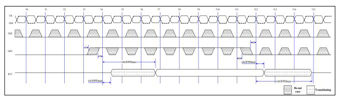
In Precharge Power Down, ODT receiver remains active; however no Read or Write command can be issued, as the respective ADD/CMD receivers may be disabled.
