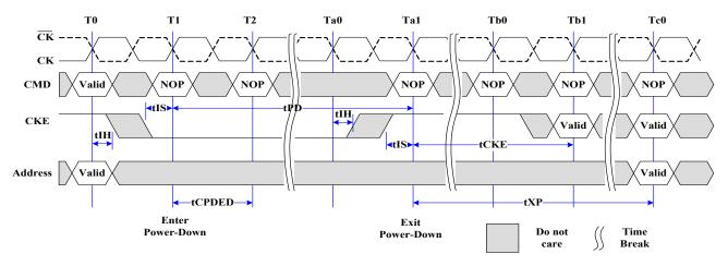
Timing Diagrams for CKE with PD Entry, PD Exit with Read, READ with Auto Precharge, Write and Write with Auto Precharge, Activate, Precharge, Refresh, MRS:
