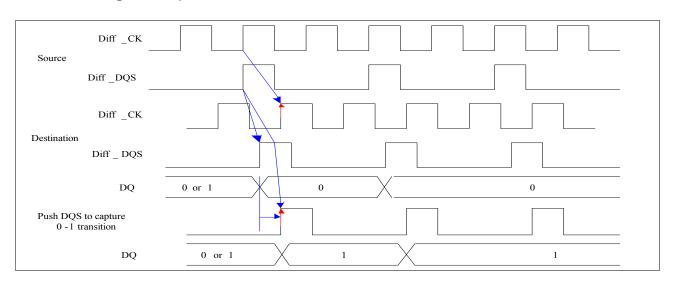
DQS/DQS driven by the controller during leveling mode must be determined by the DRAM based on ranks populated. Similarly, the DQ bus driven by the DRAM must also be terminated at the controller.
