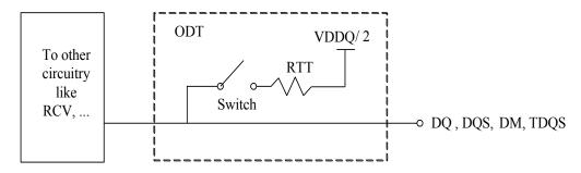
The switch is enabled by the internal ODT control logic, which uses the external ODT pin and other control information. The value of RTT is determined by the settings of Mode Register bits. The ODT pin will be ignored if the Mode Register MR1 and MR2 are programmed to disable ODT and in self-refresh mode.
