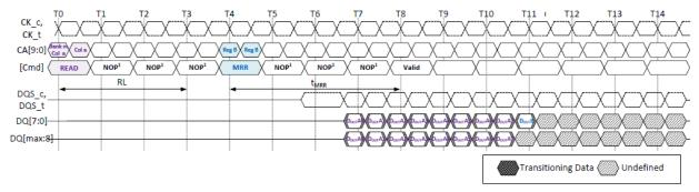
NOTE 1 The minimum number of clock cycles from the burst READ command to the MRR command is BL/2.
