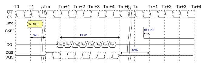
NOTE 1 CKE can be registered LOW at WL + 1 + BL/2 + RU(tWR/tCK) clock cycles after the clock on which the WRITE command is registered.
