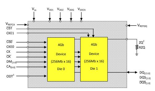
NOTE 1 ODT will be connected to rank0 (die0). The ODT input to rank1 (die1) will be connected to VSS in the package.
