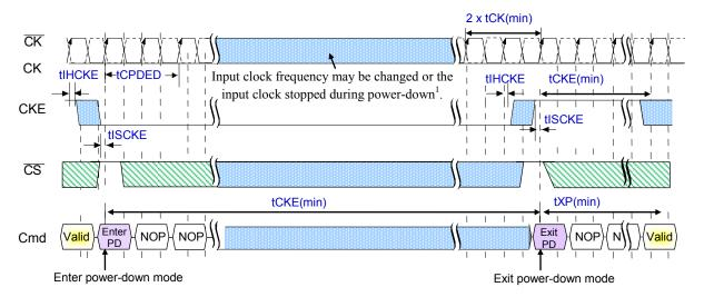
NOTE 1 Input clock frequency can be changed or the input clock can be stopped or floated during power-down, provided that upon exiting power-down, the clock is stable and within specified limits for a minimum of 2 clock cycles prior to power-down exit and the clock frequency is between the minimum and maximum specified frequency for the speed grade in use.
