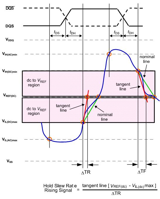
Hold Slew Rate Falling Signal =  $\frac{\text{tangent line }[V_{\text{IH(dc)}}\text{min - }V_{\text{REF(dc)}}]}{\Lambda \text{TF}}$
