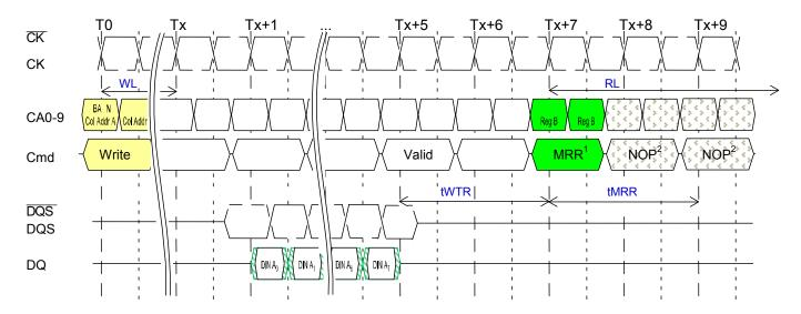
NOTE 1 The minimum number of clock cycles from the burst WRITE command to the MRR command is [WL + 1 + BL/2 + RU(tWTR/tCK)].
