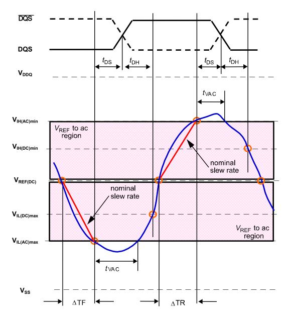
Setup Slew Rate Falling Signal =
