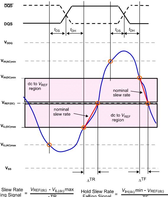
Hold Slew Rate Falling Signal =
