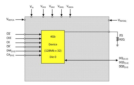
NOTE 1 ODT pin is NOT supported. ODT die pad is connected to VSS inside the package.
