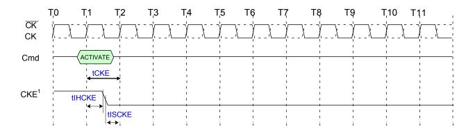
NOTE 1 CKE can go LOW tIHCKE after the clock on which the ACTIVATE command is registered.
