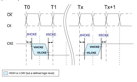
NOTE 1 After CKE is registered LOW, CKE signal level shall be maintained below VILCKE for tCKE specification (LOW pulse width).
